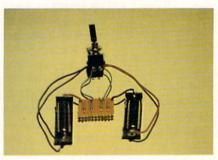
Photo 2. Power supply completed with batteries.
